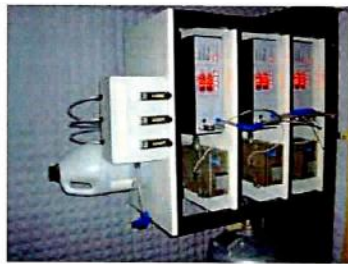
Parker nitrogen compressor _____ RH control units RK2 _____ Pressure tank
